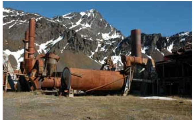
2.2 The rotary guano cookers on the south side of Building No. 2
