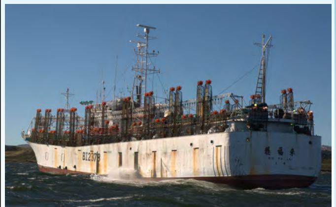
Figure 5.15 A typical jigging vessel.
