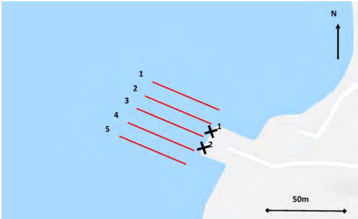
Figure 31. KEP wharf showing 5 (1-5 red lines) video survey tracks and 2 (1&2 black crosses) vertical wharf surveys
