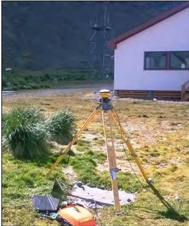
Figure 4-3; Position logging on ISTS-61.
