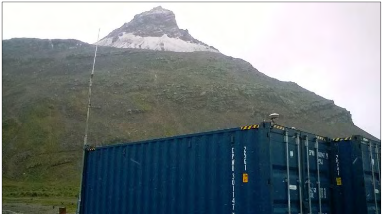
Figure 4-2; RTK base set up on the container.
