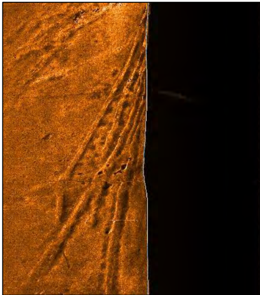
Figure 3-3; Anchor marks in the seabed (only port channel shown).
